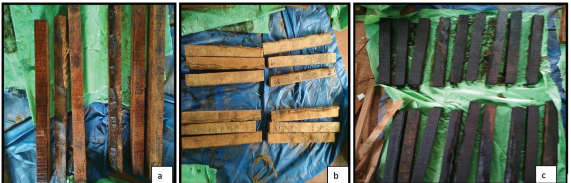
Figure 1. (a) Wood samples treated with neem oil (b) Wood samples treated with turpentine (c) Wood samples treated with CNS liquid
