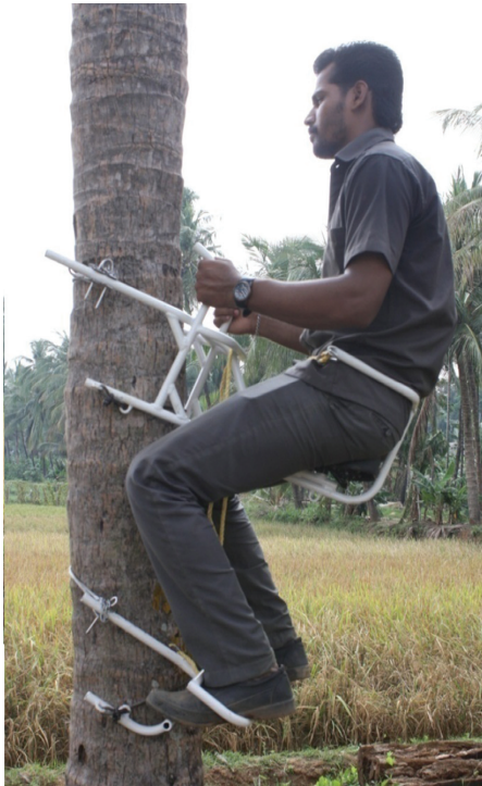
Plate 2. Operational view of developed coconut palm climbing device
