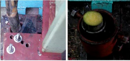
Plate 3 Specimen in impact test rig before and after cut
