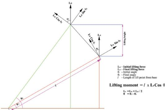
Figure 2. Schematic representation of lifting moment calculation
