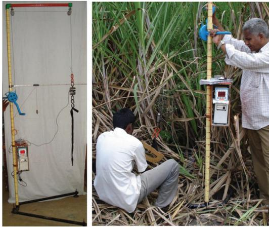
Plate 1. Lifting force measuring apparatus and its field measurement
