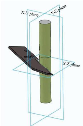
Figure. 6 Position of cutting blade showing tilt and oblique angles with respect to the co-ordinate planes
