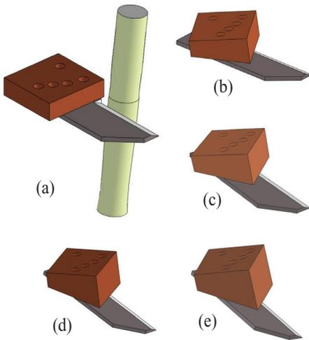
Figure. 8 Angled wooden blocks blade at different Tilt and Oblique angles
