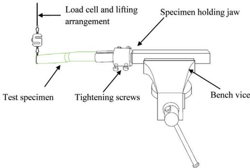
Figure 4. Schematic of experimental set up for measuring modulus of elasticity using cantilever bending test
