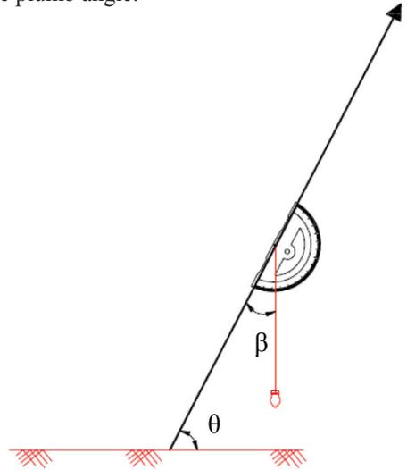
Figure 1. Measurement of degree of lodging of sugarcane
