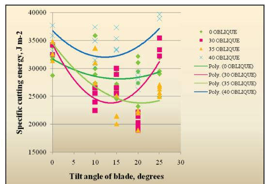
Figure. 11 Specific cutting energy Vs Tilt angles for different Oblique angles
