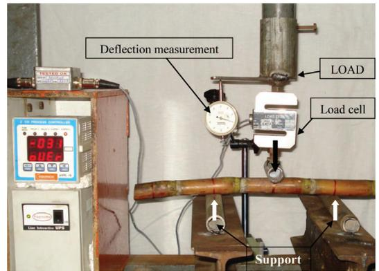
Plate 2 Set up for measurement of modulus of elasticity using simple supported beam
