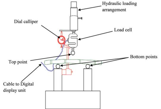
Figure 3. Schematic of experimental set up for measuring modulus of elasticity using simple supported bending test
