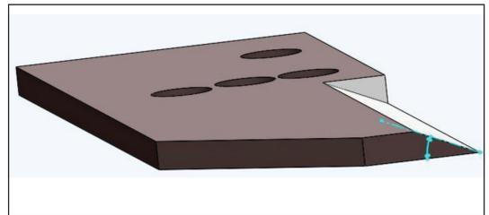
Figure 5 Measurement of bevel angle of blade cutting edge
