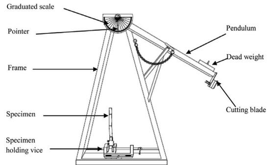
Figure. 7 Schematic of pendulum type impact test rig.
