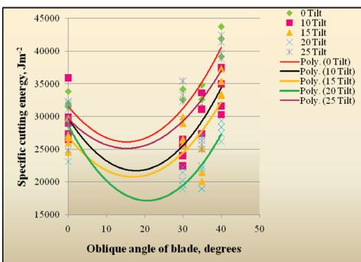
Figure. 10 Specific cutting energy Vs Oblique angles for different Tilt angles
