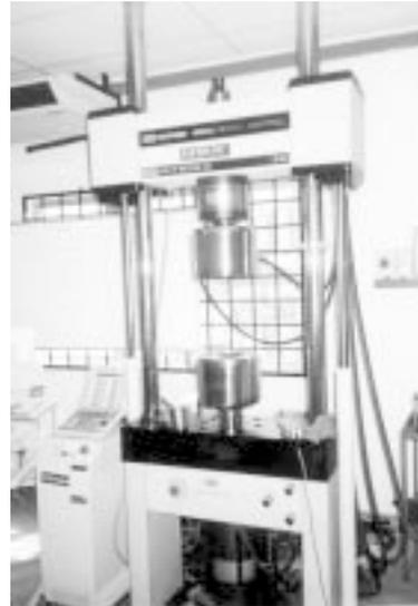
Fig. 2: The test set-up: INSTRON 3142 Dynamic Material Testing System (INSTRON Industrial Products, Grove City PA, USA)
