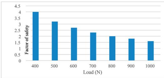
Figure 11. Factor of Safety w.r.t applied loads of the top frame of the climber
