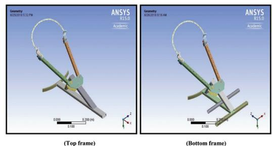
Figure 4. Three dimensional models of the climber
