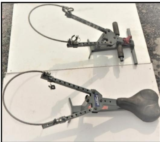
Figure 3. Farmer's model of a 'Sit and stand type coconut climber
