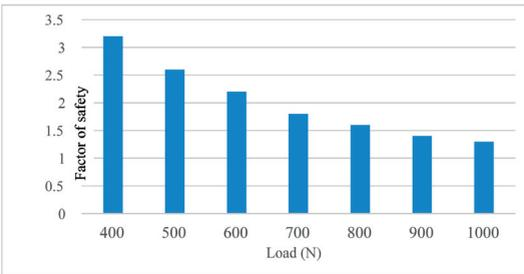
Figure 12. Factor of Safety w.r.t applied loads of the bottom frame of the climber
