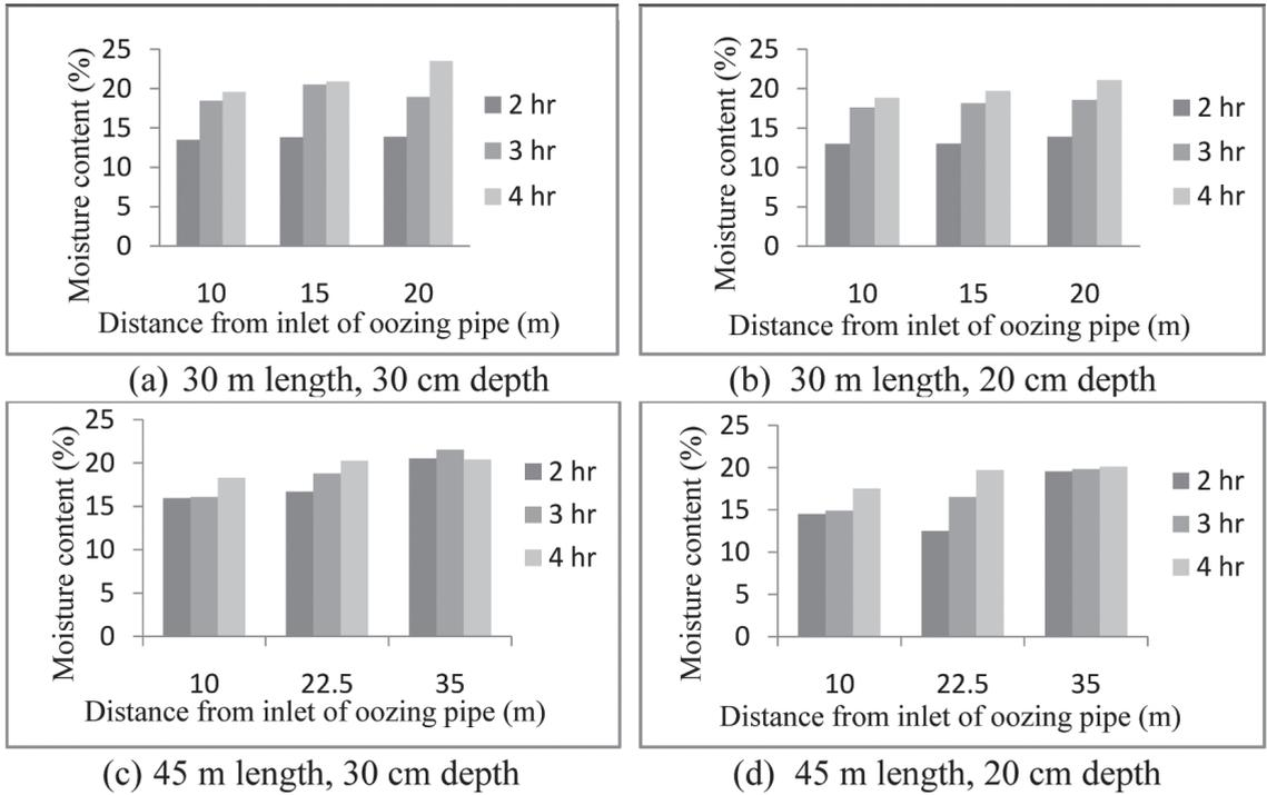
Figure 2. (a) to (d). Average soil moisture content observed under different combinations of selected lengths and depths for 2, 3 and 4 hours of operation of irrigation
