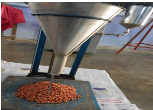
Figure2. Measurement of angle of repose
