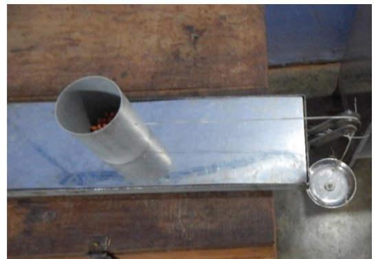
Figure 3. Measurement of angle of internal friction
