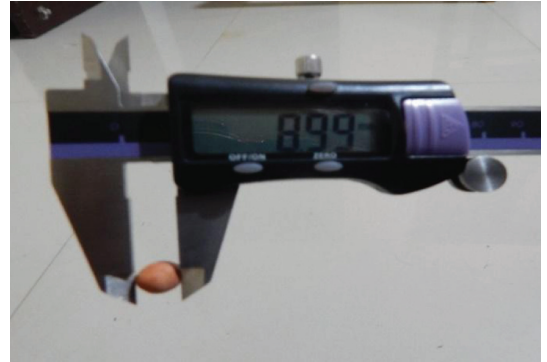
Figure 1. Measurement of axial dimensions of the groundnut seed
