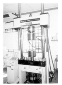
Fig. 2: The test set-up: INSTRON 3142 Dynamic Material Testing System (INSTRON Industrial Products, Grove City PA, USA)
